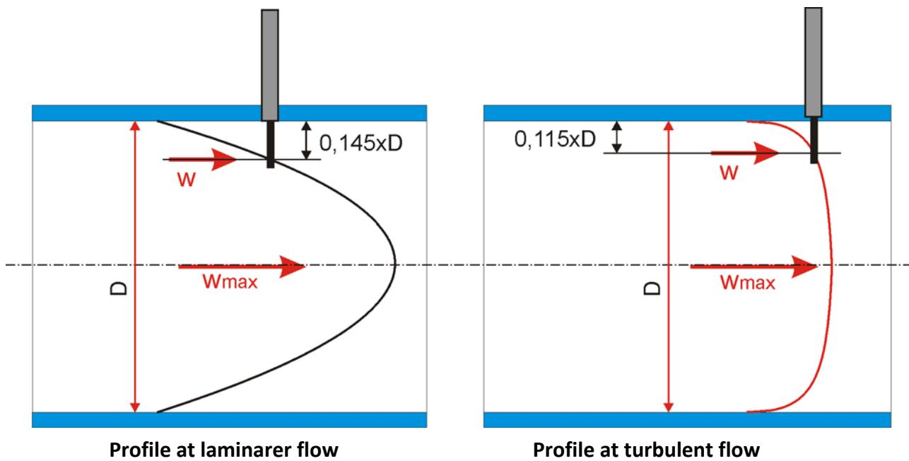
A constant undisturbed flow profile has a radius around the centre line of pipe where the averaged flow velocity may be measured.
