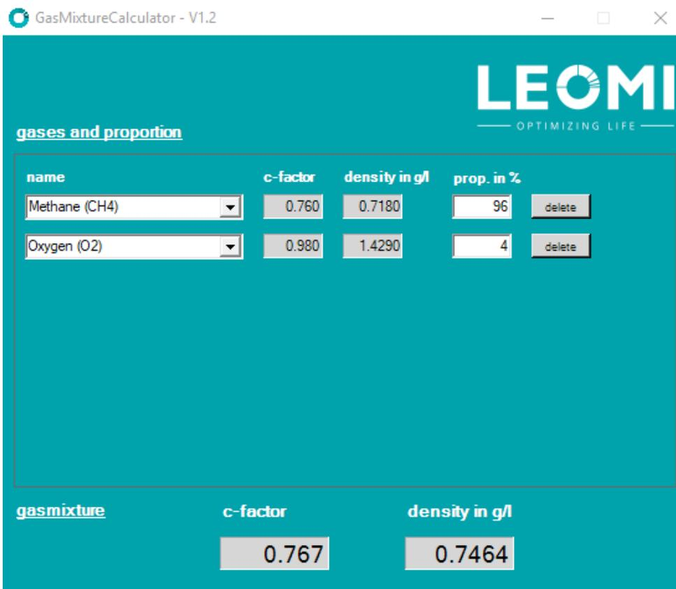
Note: This calculator is for Leomi-586 and Leomi-587 insertion thermal mass flow meters model.
